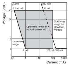
The above diagram is for standard conditions (5°C to 35°C, 40% to 70%). Since the values vary depending on the operating environment conditions, contact your OMRON representative for further details.
