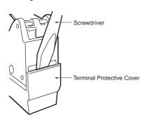
When mounting the Terminal Protective Cover to the case, align the cover on the case and then press the cover down to mount it firmly. If the cover is pressed down in an inclined position, rubber packing will deform and thus affect the sealing capability.
